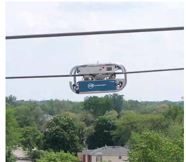
Exelon has partnered with Prysman Group to pilot Prysman's E3X ® Robot System that is designed to apply heat-dissipating coatings to existing power lines to enhance transmission efficiency and safety.
