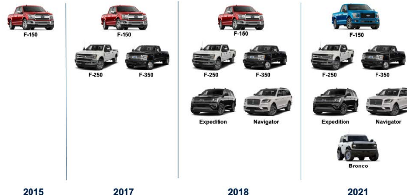
The F-150, F-250, F-350, Expedition and Navigator have all aluminum vehicle bodies. The Bronco has aluminum doors, swing gate, hood and fenders.
