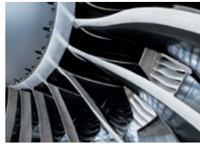
With the GE90, GE introduced the composite fan blade—the first-ever in commercial aviation.
