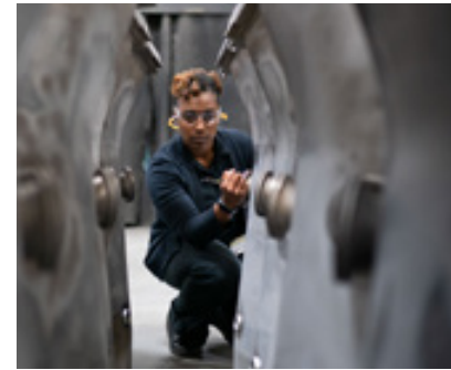
Wysheka Austin inspecting 7HA.02 Gas Turbine unibody
