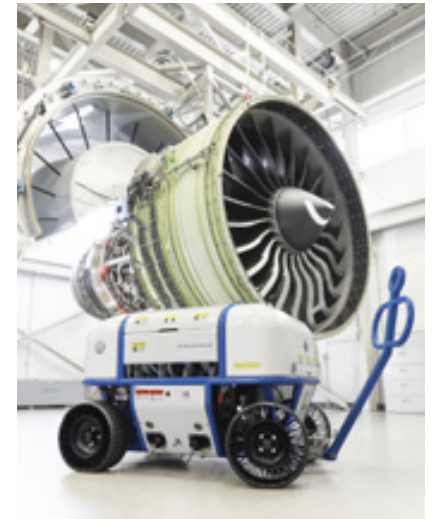
GE's proprietary detergent solution 360 Foam Wash has more cleaning capability than typical water wash. The process involves injecting a specially-formulated, proprietary solution that removes dust and dirt particles in the engine.
