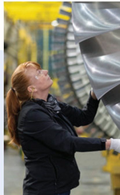
Vicki Lunsford helps build the heart of the first-ever 7HA.03 Gas Turbine, the rotor, for Florida Power & Light.
