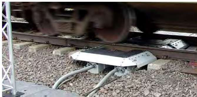
Wheel profile detectors capture critical information every time a train passes by.
